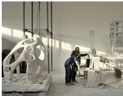
3D printer designed by E. Dini, capable of creating buildings from stone
